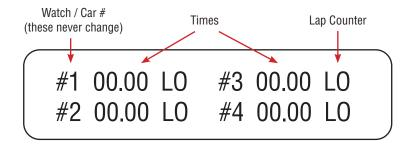
**TO USE THE STOPWATCH FUNCTION:** Use buttons #1 to 4 (pyrometer Memory) for timing. These correspond to #1 to #4 on the display.
